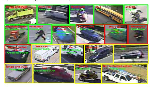
Fig. 6: Classified images from the validation dataset using EDeN. The red text is the ground-truth and the green text is the predicted class. The images in the green frame are correct classification, the images in the red frame are wrong classifications and the images in the yellow frame are noisy data with wrong ground-truth but EDeN predicted them correctly.
